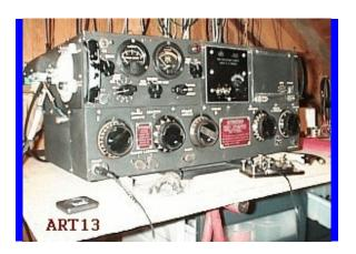
The Brooks amateur station used military style surplus equipment which was very popular in the 40-s 50s and 60's - and still in demand of today's collectors. The ART-13 Collins 813 final tube auto tune transmitter and the BC348 HF surplus receiver, (ART13 pictured) The station antenna was a half wave doublet. I can envision the doublet stretched between two pines.
